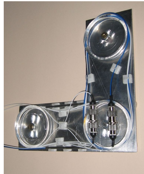
Fig. 2: Photograph of a detector showing the optical fibers forming the two orthogonal arms. See Fig. 1 for the schematic layout. The 2 \times 2 beam splitter and joiner (Thorlabs FC632-50B-FC) are the two small stainless steel cylindrical tubes. The two FC to FC mating sleeves (Thorlabs ADAFC1) are physically adjacent. The overall dimensions of the metal base plate are 160 \times 160 mm. The 2 \times 2 splitter and joiner each have two input and two output fibers, with one not used. Arm 2 is folded over the splitter and joiner, compared to the schematic layout. The interferometer shown costs approximately $400.
