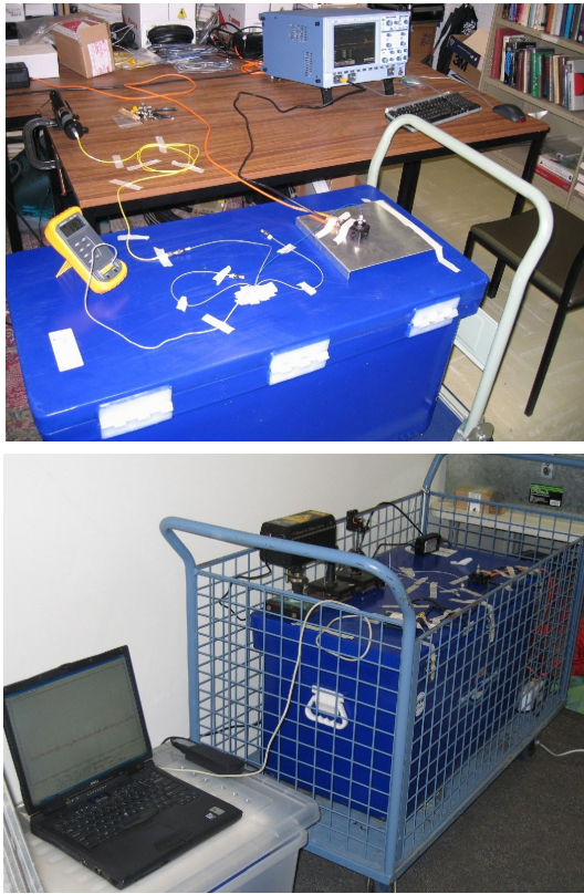
Fig. 3: (a) Detector 1 (D1) is located inside a sealed air-filled bucket inside an insulated container (blue) containing some 90 kg of water for temperature stabilisation. This detector, in the School of Chemistry, Physics and Earth Sciences, had an orientation of 5^\circ anti-clockwise to the local meridian. Cylindrical He-Ne laser (Melles-Griot 0.5 mW 633 nm 05-LLR-811-230) is located on LHS of bench, while data logger is on RHS. Photodiode detector/pre-amplifier is located atop aluminium plate. (b) Detector 2 (D2) was located 1.1 km North of D1 in the Australian Science and Mathematics School. This detector had an orientation of 11^\circ anti-clockwise to the local meridian. The data was logged on a PC running a PoScope USB DSO (PoLabs http://www.poscope.com ).
