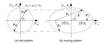
Fig. 1: Binary light flash systems whose centers of inertia are (a) at rest (b) moving at speed  $V = \beta c$ .
