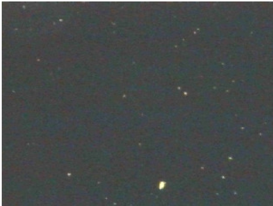
Fig. 3: The control sample of distilled water, examined using a novel microscope technique. It looks mainly black because there are no “structures” or domains to reflect the light, apart from a bit of noise (e.g. from ambient lighting).
