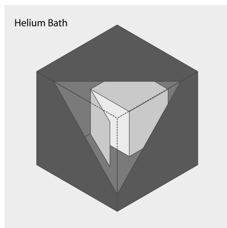
Fig. 1: Schematic representation of our thought experiment. A large outer cavity acts as an ideal blackbody ( \epsilon = 1 , \rho = 0 ) and is initially immersed in a helium bath at 4 K. Within this cavity, a perfectly reflecting enclosure ( \epsilon = 0 , \rho = 1 ) rests on the floor with one of its sides initially remaining open.
