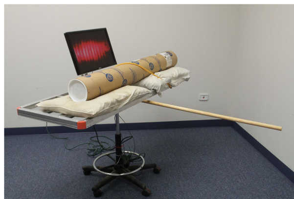
Fig. 13: Complete system with vibrational and thermal mitigation.
