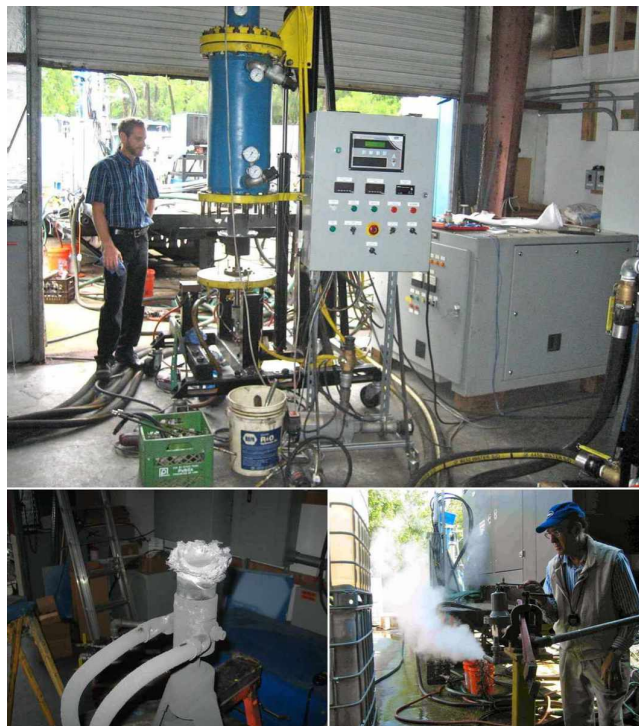
Fig. 8: In this figure, we show the Oxygen hadronic reactor for the ICNF of Helium and Carbon into Oxygen (Sect. 4.5) with the structure outlined in Fig. 5, including: in the top view, the engineer Chris Lynch, the reactor, its control panel and the power unit; in the bottom left view, the scorching of the cathode despite its continuous cooling by the flow of the Helium; in the bottom right view, the production of steam operated by the author.
