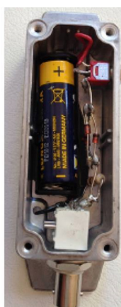
Fig. 1: Left: Circuit of Zener Diode Space Flow Detector, showing a 1.5 V AA battery, two 1N4728A Zener diodes operating in reverse bias mode, having a Zener voltage of 3.3 V, and resistor R=10\text{ k}\Omega [2].
