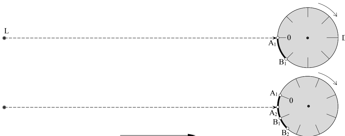
Fig. 4: Schematic of the experimental set-up: A 1 and A 2 denote the points where the rays generated by the first and the second light pulse hit the disk D at the instants t 1 and t 2 . The circular arc length A 1 B 1 = d represents the trace on D’s photosensitive lateral surface the very first pulse causes. B 1 B 2 = ωδt A depicts the trace’s length increment produced by the second and any additional pulse according to the propagation hypothesis. The arrow at the bottom indicates the direction of motion of the earth around the sun.
