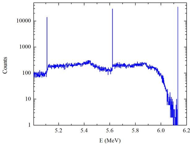
Fig. 6: Calculated spectrum in the 300 cc detector from a Teflon shield of 5cm.
