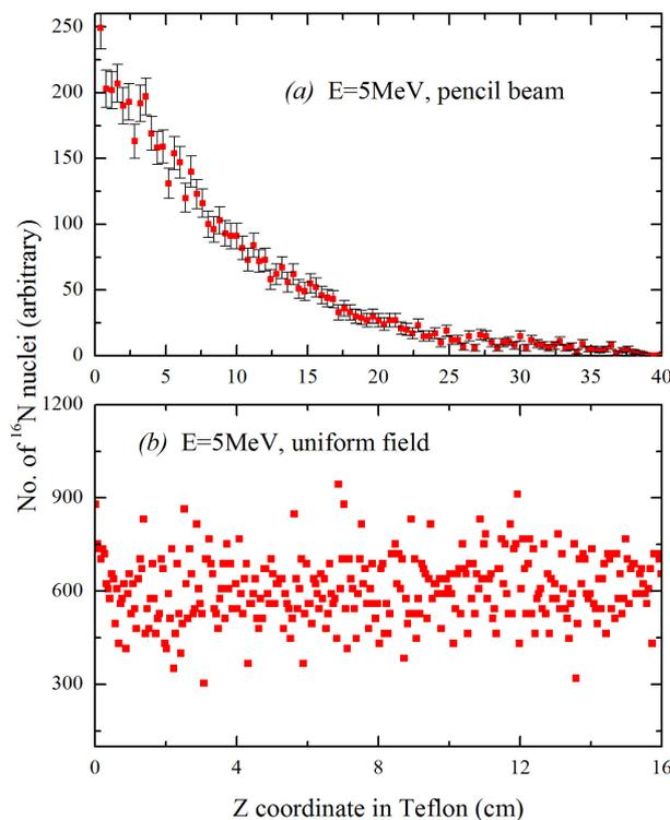
Fig. 4: The distribution of the  $^{16}\text{N}$  nuclei along the  $z$  axis of the Teflon cylinder for two cases: (a) pencil beam and (b) uniform flux. In the second case the standard deviation is larger (17%) but the distribution is undoubtedly uniform.
