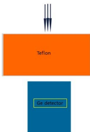
Fig. 1: A pencil neutron beam is hitting few cm thick Teflon absorber, at 5.0 mm above a  $\phi$  64 $\times$ 90 mm Ge coaxial detector, placed in a 1 mm thick Aluminum case (not shown).
