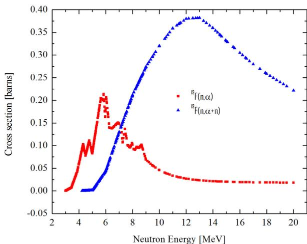
Fig. 2: The cross sections of the  $^{19}\text{F}(n,\alpha)$  and  $^{19}\text{F}(n,\alpha+n)$  reactions taken from the Japanese cross sections library JENDL-4.0.
